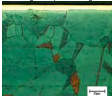
Fig. 2. AISI 316L nitrided at 400°C (752°F); Fig. 3. AISI 316L nitrided at 450°C (842°F); Fig. 4. AISI 316L nitrided at 500°C (932°F)
